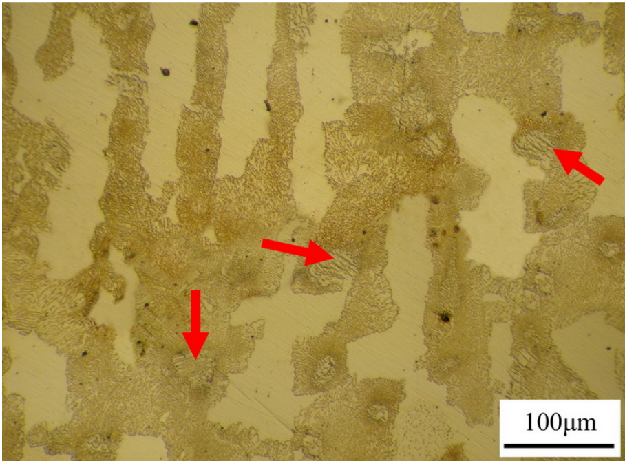
Figure 4. Formation of pearlite-like structure in the cross section of failed roller. The arrows show the large pearlite-like colonies.
