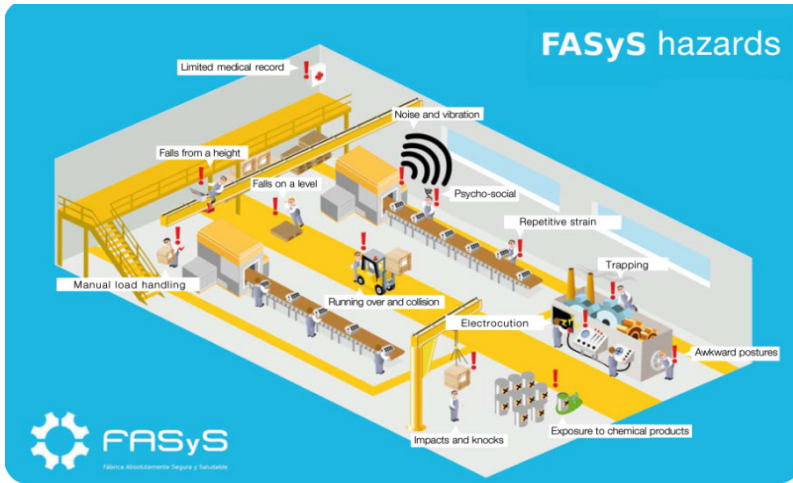
Figure 2. FASyS 13 prevalent hazards
