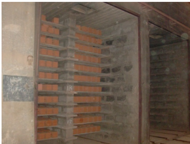
Figure 7. Brick drying compartment
