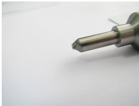
Figure 10. Mixing head needle corrosion by EG
