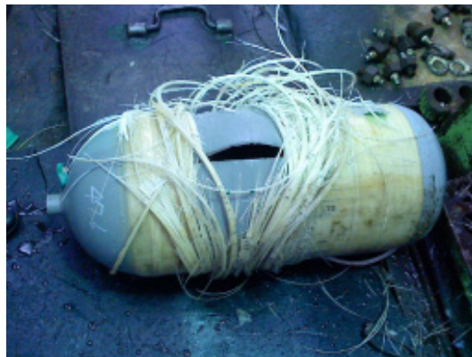
Figure 4. Composite vessel after burst test
