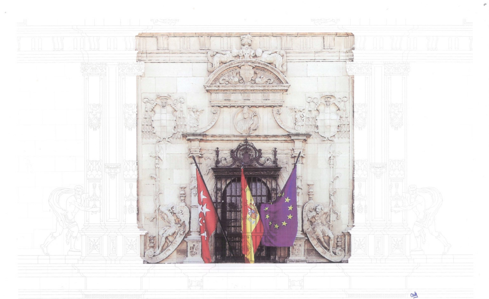
Figure 5. Accurate drawing of the 16 th century façade of the Colegio de San Ildefonso (Alcalá de Henares, Spain), using photogrammetrical techniques (Task Group's Partner: Cultural Heritage and sustainable architecture Research Team , University of Alcalá, Spain).
