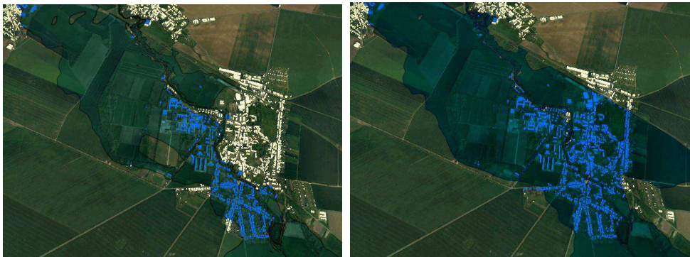
Fig. 13. Simulation of affected areas (blue) and not affected areas (white) during a flood 1994 (right); simulation with planned dams (right) (Buhmann & Pietsch, 2008a)
