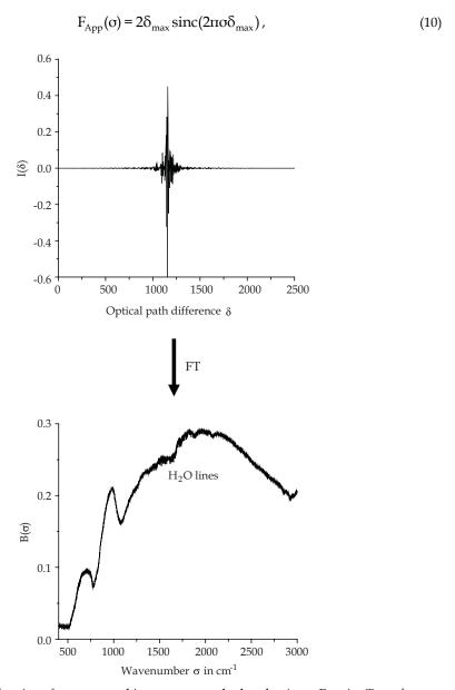
Fig. 2. Example of an interferogram and its spectrum calculated using a Fourier Transform algorithm
