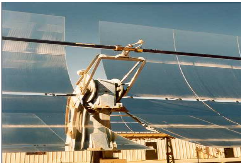
Fig. 2. Typical solar collector-receiver subsystem
