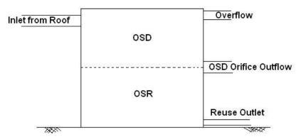
Fig. 3. Rainwater tank with inlet, overflow, outlet and optional third outlet for detention control.
