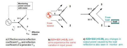
Fig. 5. Benefits by inserting coaxial power splitter
