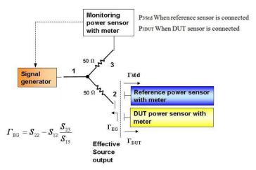
Fig. 4. Coaxial splitter based power measurement setup
