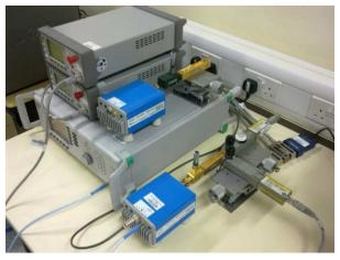
Fig. 12. Rectangular waveguide power sensor calibration system setup
