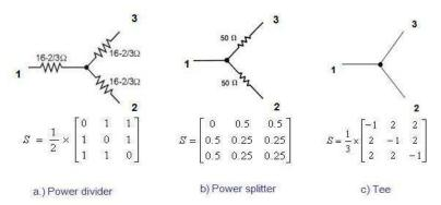
Fig. 3. Three 3-port components and their corresponding scattering parameter matrix
