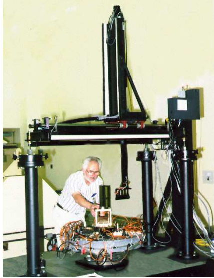
Fig. 7. Vertical Scan LTP (VSLTP) at Marshall Space Flight Center set up for measuring x-ray telescope mirrors and mandrels in the vertical orientation
