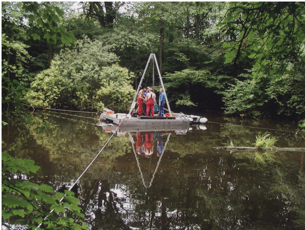
Photo 1. Morasko crater B (second in size) – obtaining cores from the bottom sediments. GeoForshungsZentrum equipment.
