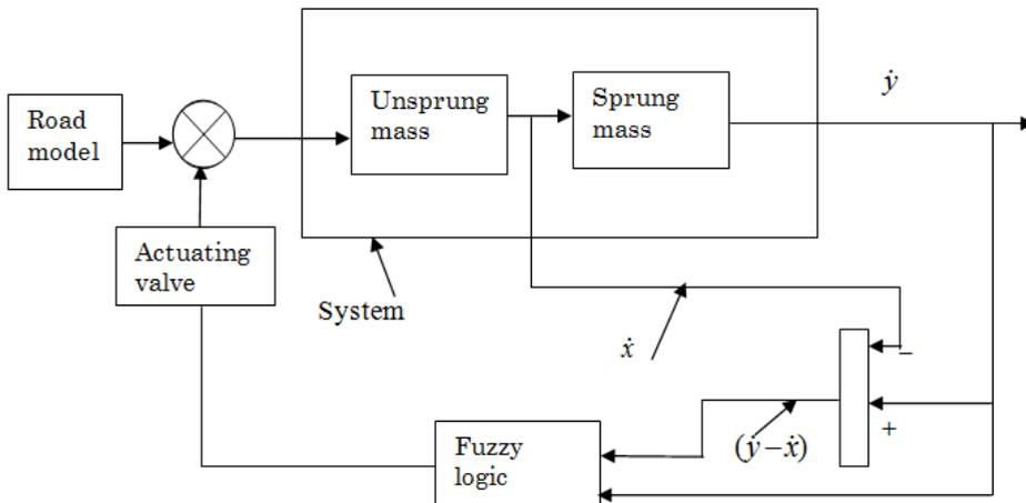
Fig. 6. Block diagram representation of the control system
