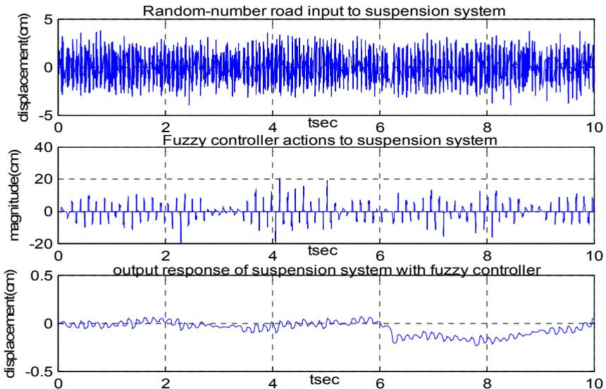
Fig. 12. Suspension controller response with random number input
