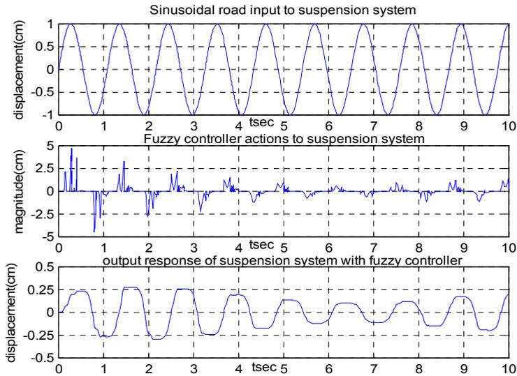
Fig. 9. Suspension controller responses with sinusoidal input
