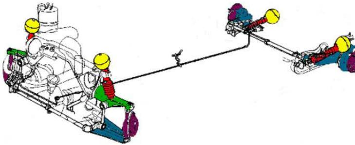
Fig. 2. Active suspension system's oil/air connection diagram
