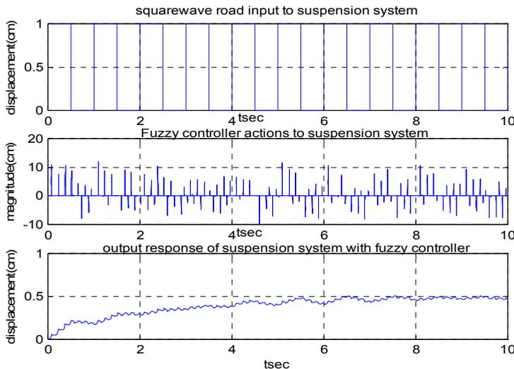
Fig. 10. Suspension controller responses with square-wave input
