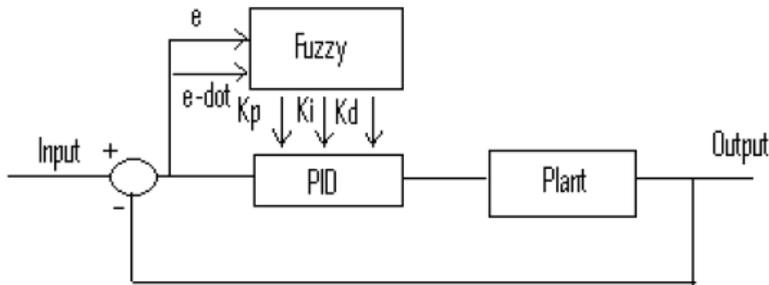
Fig. 15. Structure of the Fuzzy-tuned PID controller
