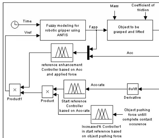
Fig. 23. Block diagram of the second scheme controller.
