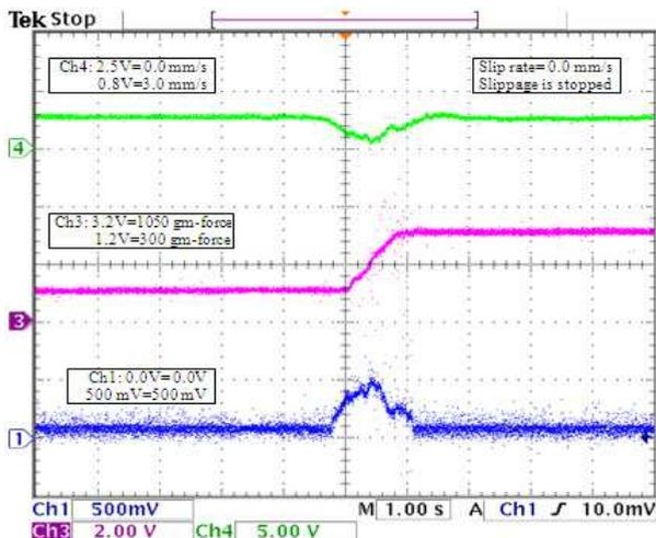
Ch4: Slip-rate (mm/s) - Ch3: Fapp (gm-force) - Ch1: Vref (V)
