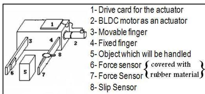
Fig. 4. Gripper configuration.
