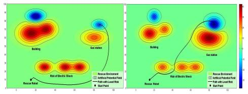
Fig. 12. Generated path for the first scenario: (a) cold and rainy condition, (b) hot and dry condition
