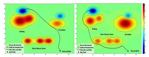
Fig. 13. Generated path for second scenario: (a) cold and rainy condition, (b) hot and dry condition
