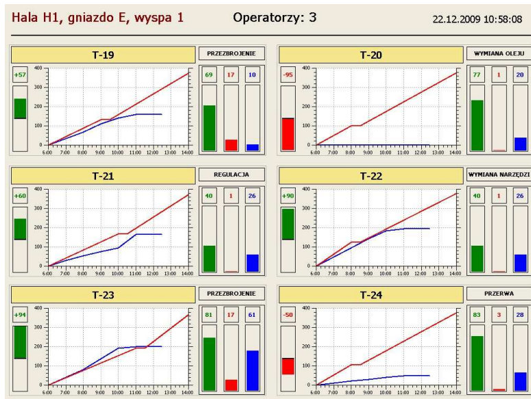
Fig. 5. The factory floor HSI locked mode screen for six machines
