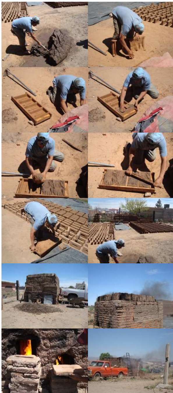
Fig. 1. Brick fabrication process at Nuevo Casas Grandes, Chihuahua.
