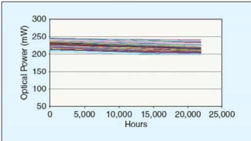
Fig. 6. Monitored lifetest data for a x64 element array operating at 8xx nm. The array module exhibits highly robust performance over 20,00 hour CW operation.
