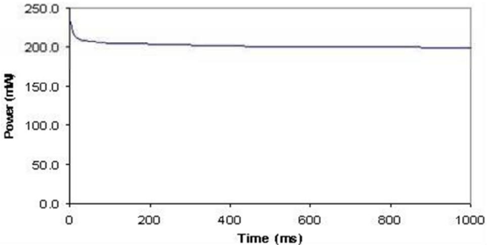
Fig. 12. Measured power-droop across fully packaged array module.
