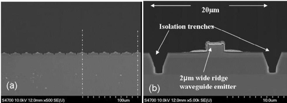
Fig. 9. SEM images of a  $20\ \mu\text{m}$  pitch red laser array, showing (a)  $\times 500$  magnification of half the array chip, (b)  $\times 5000$  magnification of a single emitter within the array.
