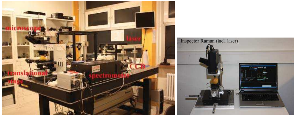
Fig. 2. The Raman equipment at The Molecular Sensing Engineering group at Faculty of Engineering, Institute of Technology and Innovation, University of Southern Denmark. (a.) The Raman setup, which is suited for scientific purposes. The Raman spectrometer is combined with an optical microscope, which is equipped with a motorized XY-stage on the translational stage. (b.) A portable commercial Raman setup: DeltaNu Inspector Raman, 785 nm excitation, unpolarized Raman, spectral resolution: 10, 12 or 15 \text{cm}^{-1} , predefined laser power 1.8, 3.4 and 6 mW, polystyrene standard for wavelength calibration, battery operated. Inspector Raman has been equipped with a manual translational XY-stage, order to be able to translate the laser across the sample.
