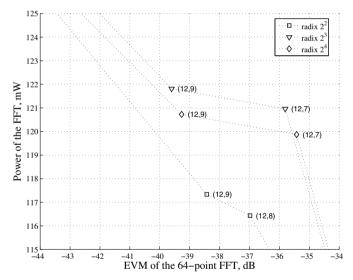
Fig. 10. EVM and power of the pipeline–SDF DIF 64–point FFT/IFFT core 2003) proposes a normalization of the power consumption as,
