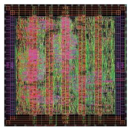
Fig. 12. Layout of the 64 complex–point FFT/IFFT fabricated in a 90 nm technology, 6–ML CMOS process. The core size is  $0.370 \times 0.368~mm^2$
