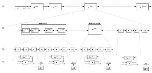
Fig. 1. Structure of typical stages of  $r^k$  pipeline SDF architectures
