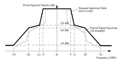
Fig. 3. Spectral mask of a transmitter output
