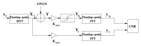
Fig. 6. System model to estimate the CNR for different values of  $K_{AGC}$
