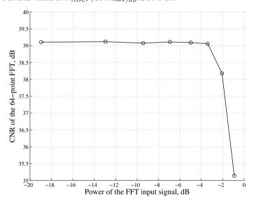
Fig. 7.  $(CNR)_{dB}$  vs the power of the input signal in the FFT  $(P_{Y_a})$
