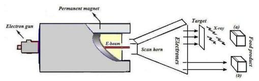
Fig. 2. Schematic diagram of a typical x-ray (a) and E-beam (b) irradiators
