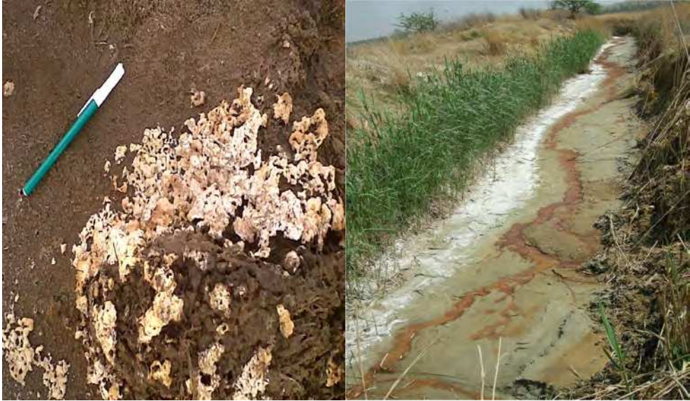
Fig. 9. Efflorescent crusts (from the top left in a clockwise direction): at a tailings footprint precipitates on the wall and base (floor); distinct white and yellowish precipitates along a flow path from the footprint; pinkish lumps of precipitates; and precipitates along a stream draining from a TSF (distinct Fe precipitates along the stream can be seen).
