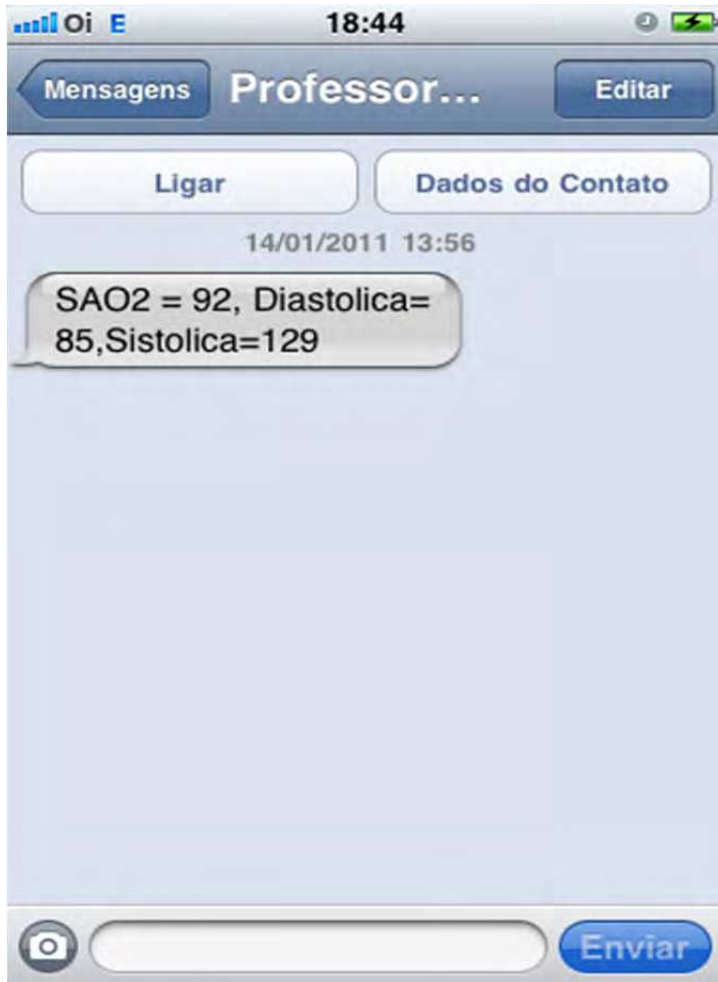
Fig. 13. Oxymeter and blood arterial pressure data sent to a cell phone via GSM communication.
