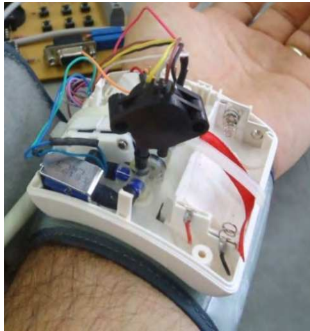
Fig. 11(a). Arterial pressure Prototype for arterial pressure acquisition.
