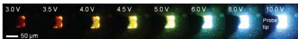
Fig. 12. Color tunability varying the voltage in a PFO-QD (70-30) based emissive film. Source: (Hong et al., 2011).
