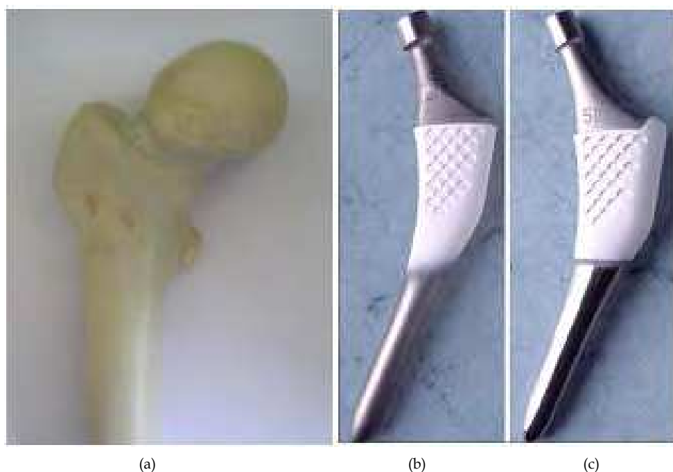
Fig. 9. Material for the development of finite element model: a) Healthy femur; b) ABG-I stem; c) ABG-II stem
