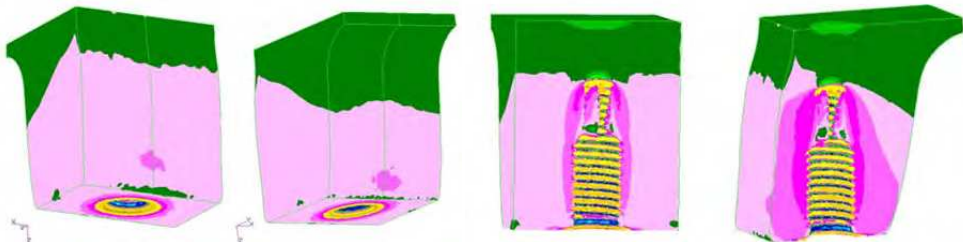
Fig. 7. Perspective and internal view of the cancellous bone. Maximum principal stresses in model under longitudinal load.
