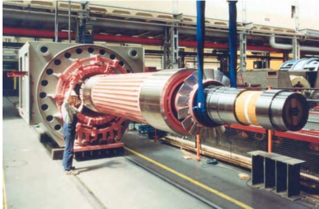
Fig. 26. Generator shaft with retaining rings, X8CrMnN 18-18 [ETE-11].
