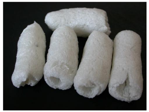
Fig. 1. Extruded starch foams.
