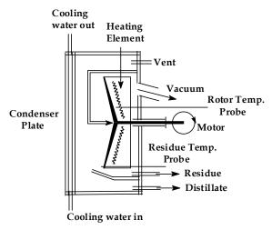
Fig. 12. Side View of Myers Pilot-15 Distillation Chamber
