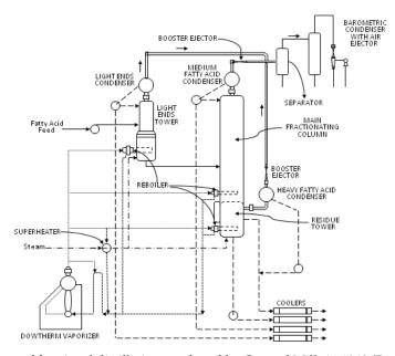
Fig. 6. Flow diagram of fractional distillation employed by General Mills in 1948 (Potts & White, 1953)
