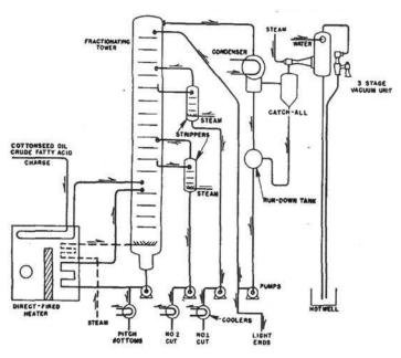
Fig. 5. Flow diagram of fractional distillation employed by Armour and Company in 1933 (Potts & White, 1953)
