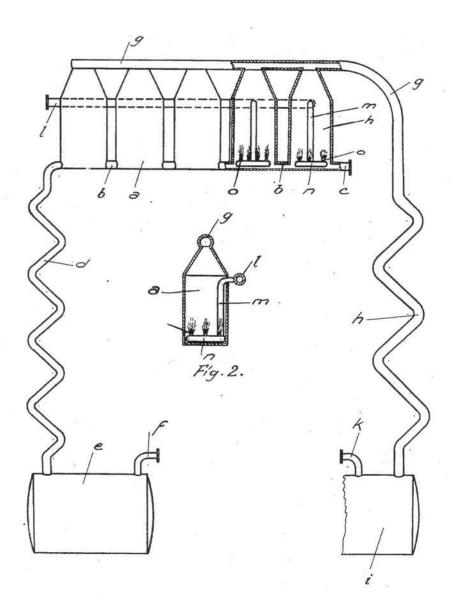
Fig. 2. Continuous distillation (Wecker, 1927)
