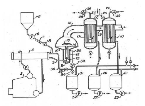
Fig. 3. Continuous dry distillation (Mills, 1942)
