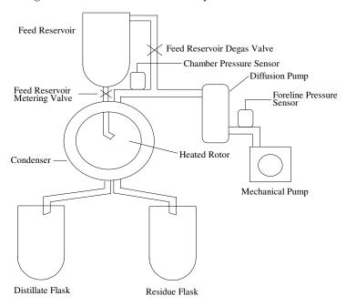
Fig. 10. Schematic diagram of Myers Lab 3 short path molecular distillation unit
