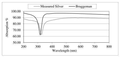
Fig. 6. Absorption vs. wavelength for 30% volume fraction silver, 160 nm thick film using Bruggeman model and a  $1.3 \mu m$  thick measured silver film.
