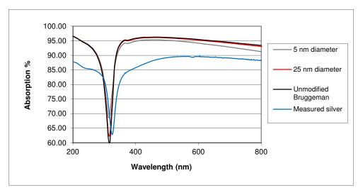
Fig. 7. Absorption vs. Wavelength for a 30% volume fraction of silver, 150 nm thick film calculated using the unmodified Bruggeman model, the Bruggeman model modified by the extended Drude model for particle diameters of 5 nm and 25 nm, and for a 1.3  $\mu$ m thick measured silver film.
