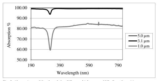
Fig. 2. Absorption vs. Wavelength for different thicknesses of V2 silver depositions.
