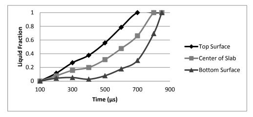
Fig. 9. Liquid Fraction vs. Time for three positions on the silver slab.
