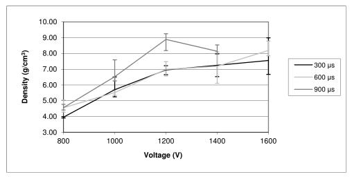
Fig. 1. Graph of Sintered Density vs. Flash Lamp Voltage.
