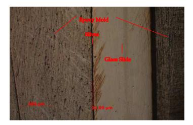
Fig. 3. Optical cross section of the V2 silver on a glass slide in an epoxy mold.
