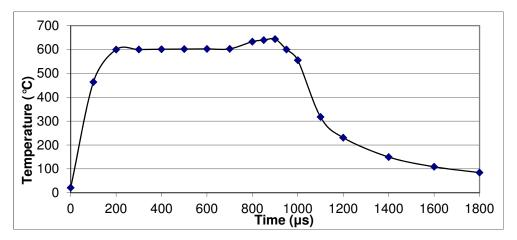
Fig. 8. Temperature vs. Time for a 10  $\mu$ m thick silver slab on a glass substrate with a flash lamp voltage of 1200V for 900  $\mu$ s.
