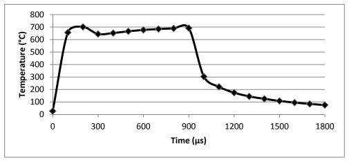
Fig. 10. Temperature vs. time for a 3  $\mu$ m thick silver slab using a 1200V flash lamp voltage and a 900  $\mu$ s pulse length using Fluent.
