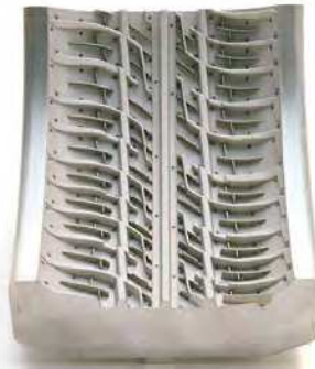
Fig. 4. Tread ring segment made by engraving on CNC.
