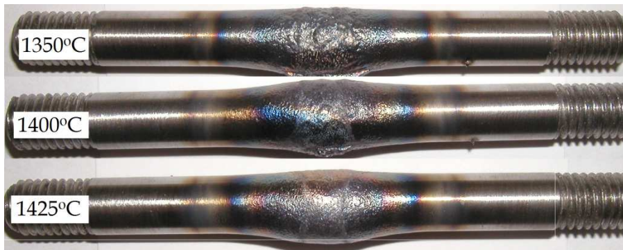
Fig. 22. Final shape of the sample after deformation at 1350°C, 1400°C and 1425°C.
