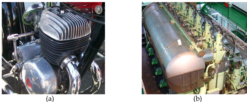
Fig. 1. (a) Spark ignition gasoline engine installed on a motorcycle. (b) Compression ignition diesel engine MAN B&W 7S50MC installed on a ship.
