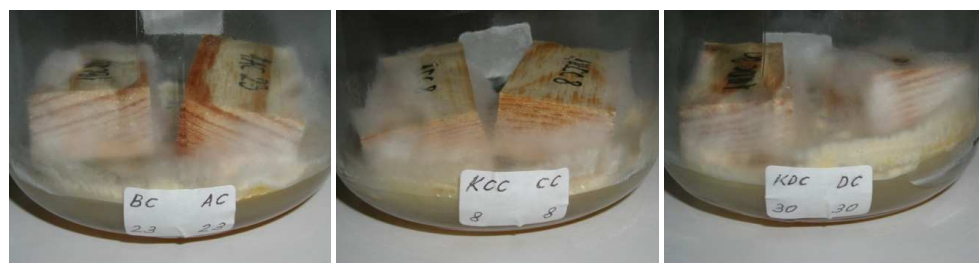
Fig. 13. Specimen pairs in testing flasks 10 days after exposure to brown-rot fungus Gloeophyllum trabeum (AC, KCC, KDC - non-irradiated controls, BC - specimen irradiated with 30 kGy, CC - 90 kGy, DC - specimen irradiated with dose of 150 kGy).
