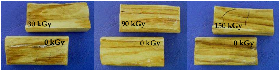
Fig. 15. Appearance of irradiated and autoclaved specimens after 16 weeks of exposure to fungus Poria placenta .
