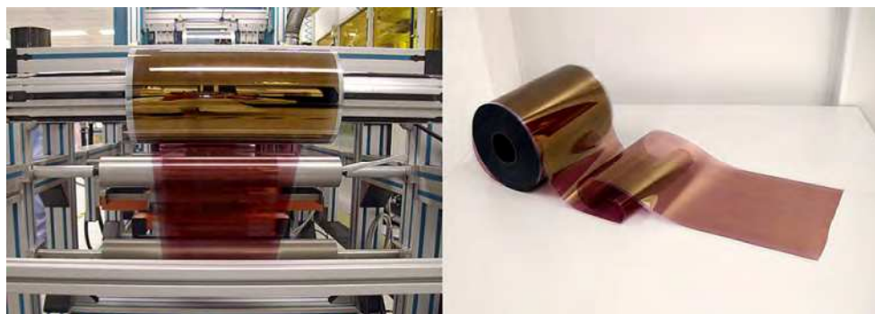
Fig. 2. Roll of the PET foil with slot die coated PEDOT and photoactive layers (reproduced with permission from (Galagan et al., 2011b), Copyright 2010, Elsevier B.V.).
