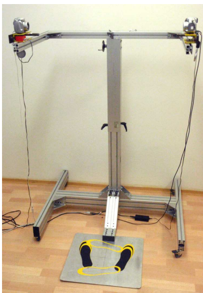
Fig. 4. The two-arm stand with fixed two cameras and laser collimators designed for the precise adjustment of the system.
