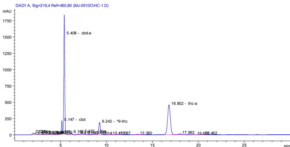
Fig. 3. HPLC (Cannabinoid) profile of a high Cannabidiol (CBD) Strain. Note the undecarboxylated THC-A and CBD-A, before heating.
