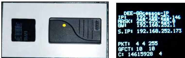
Fig. 9. EIM - System to read HID-RFID Cards.
