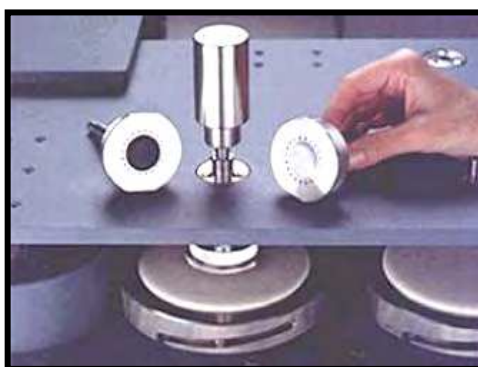
Fig. 16. Setting of sock kit on Martindale apparatus
