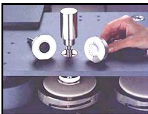
Fig. 16. Setting of sock kit on Martindale apparatus
