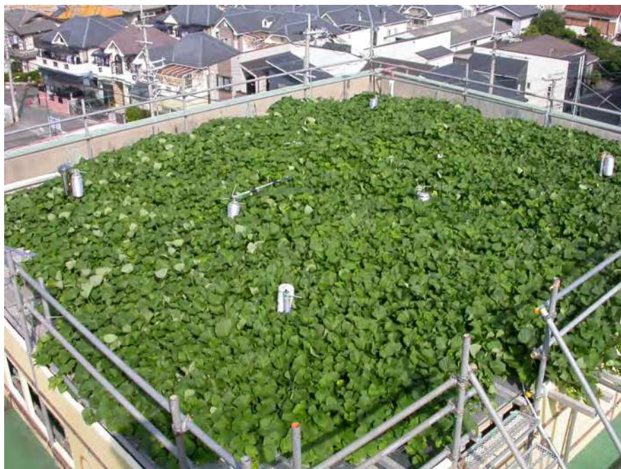
Fig. 7. Experimental system and plants growing situations at the end of September.
