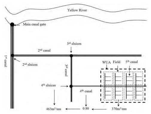
Fig. 2.3 Water allocation model for HID
