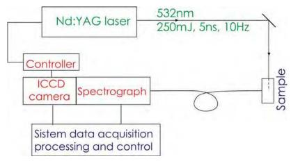
Fig. 6. The Raman spectroscopy system
