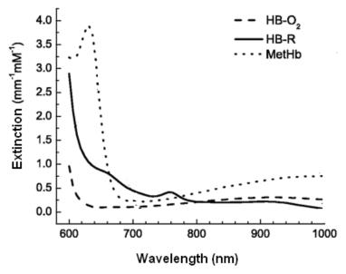
Fig. 13. The absorption spectra of hemoglobin (Hb-R), Oxihemoglobin (Hb-O<sub>2</sub>) and Methemoglobin (MetHb) (Lee et al., 2006)
