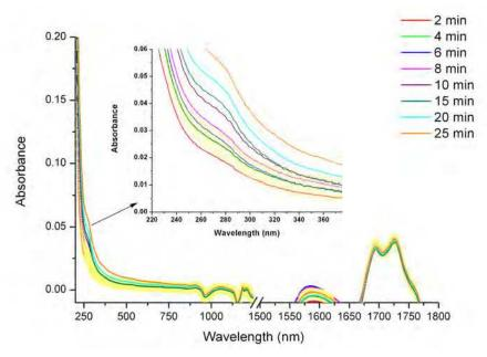
Fig. 12. The absorption spectra of Aethoxysklerol 2% exposed to 1.06  $\mu m$  Nd:YAG laser radiation.
