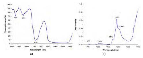
Fig. 10. The spectra of Ethanol in NIR: a) the transmission spectrum (Barun and Ivanov, 2010); b) the absorption spectrum (Smarandache et al., 2010)
