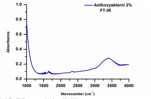
Fig. 9. The FT-IR spectrum of Aethoxysklerol 2%
