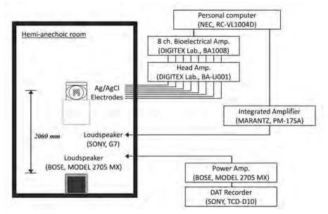
Fig. 2. Block diagram of experimental system
