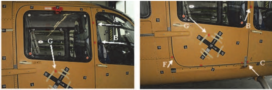
Fig. 17. Leakage points (in red) on the helicopter cabin found by means of the ultrasound technique (cabin right panels)
