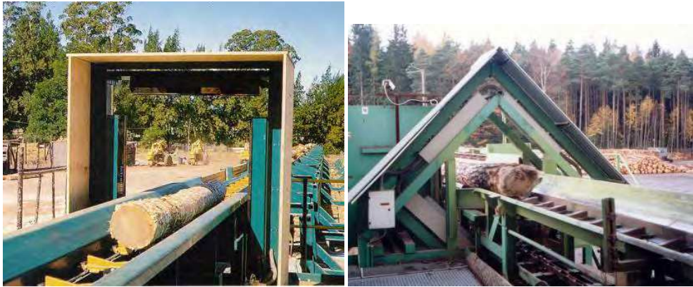
(a) vertical and horizontal position of scanning systems (b) placing the scanning systems at an angle of 45°
