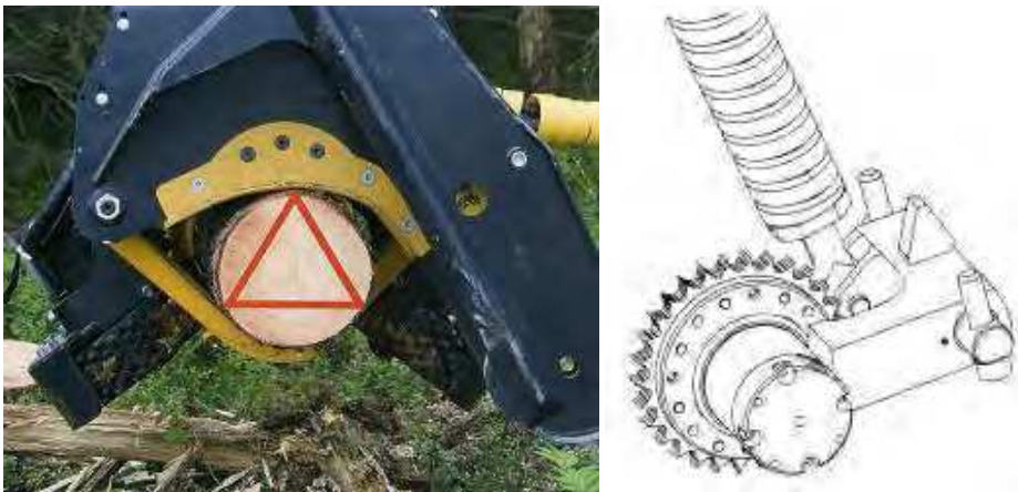
Fig. 2. Photo + scheme of scanning the stem diameter and length at harvesters (both figures according to Ponsse).
