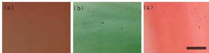
Fig. 17. Optical micrographs of drawn PVA-gold nanocomposites (4 % w/w gold, draw ratio 4): (a) unpolarized, polarization direction, (b) parallel and (c) perpendicular to the drawing direction. Scale bar is 50 mm (Park, 2006).
