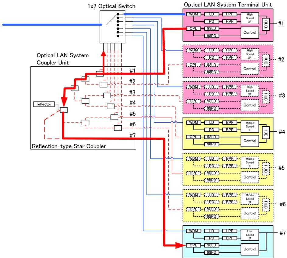
Fig. 14. Operation of communication between one “Optical LAN System Terminal Unit” and an “Optical LAN System Telephone Office Unit” using 980 nm light.
