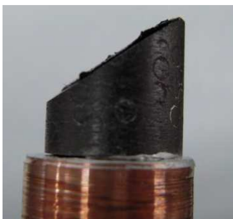
Fig. 11. Graphite anode as specimen holder.
