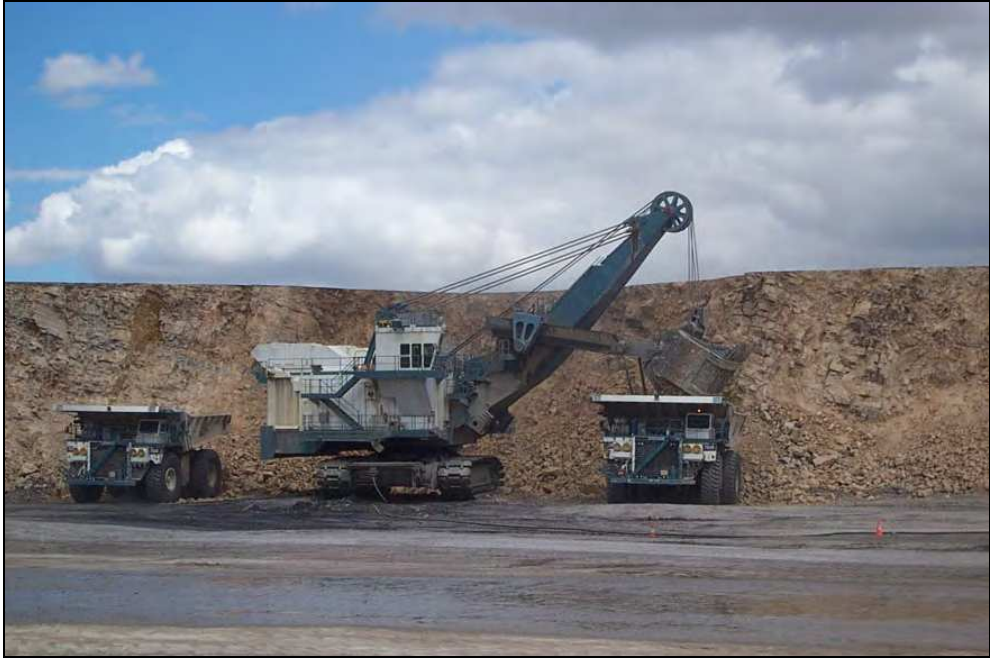
Fig. 15. Excavator removing the overburden and dumping onto trucks at Mt. Arthur Coal Mine (after Tredinnick, 2005).
